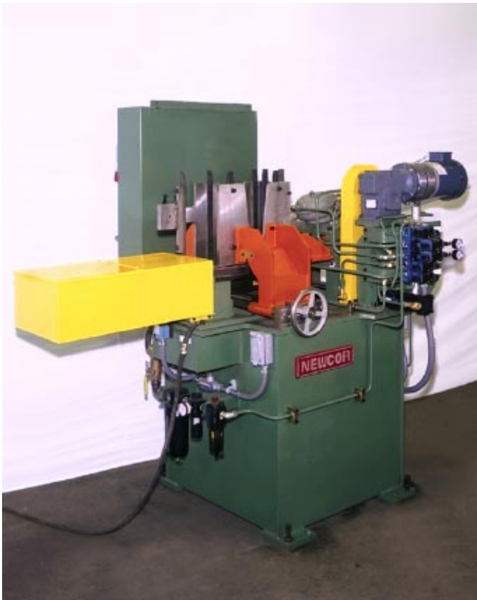
ROLL FORMER This 3-roll former automatically is fed blanks, one at a time, from a bottom feeding magazine. 9620
