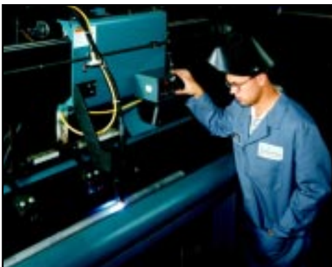
Arc / Plasma longitudinal seam welder
