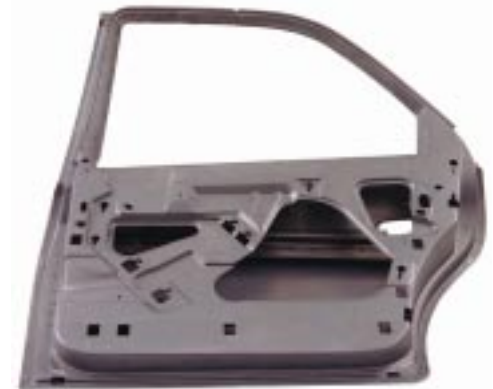
Pre-painted steel and closure panel hems
